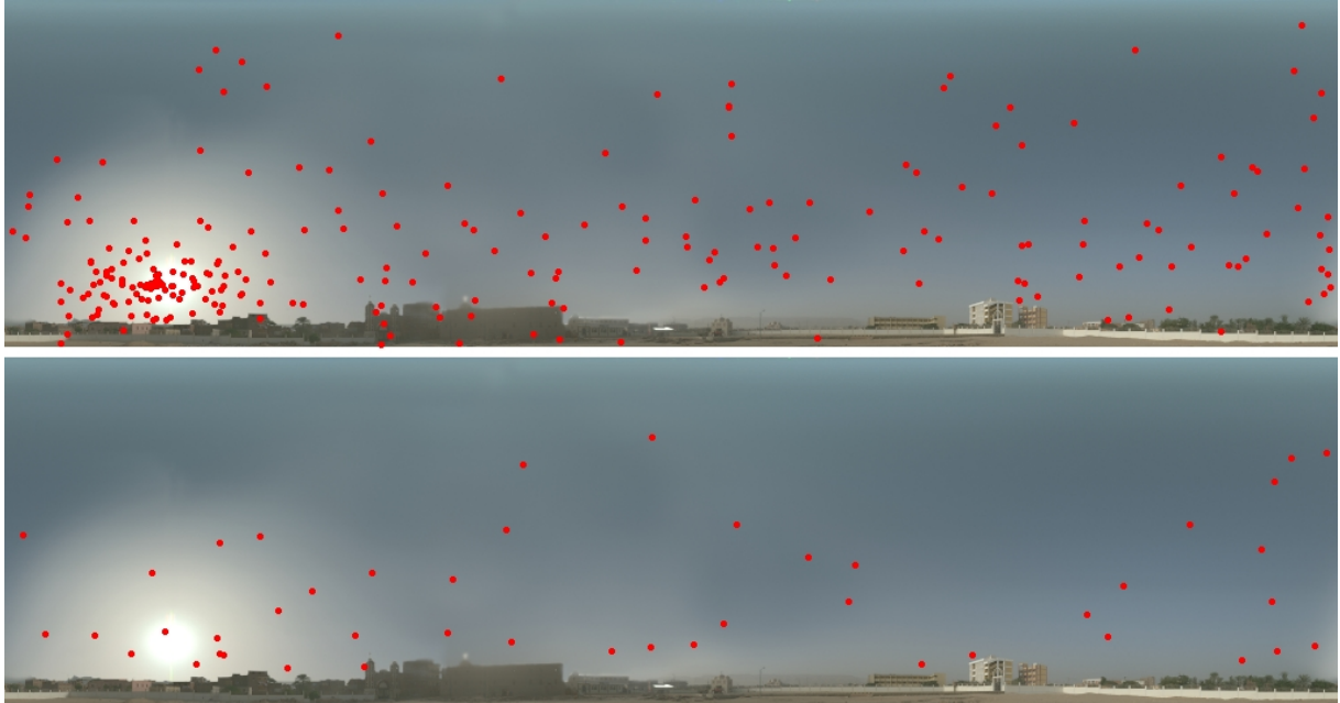
Figure 1: Top: Importance sampling of frame with 256 samples. Bottom: Light positions after clustering of samples using 56 clusters.
