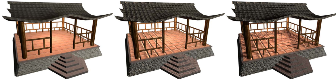
Figure 1: Japanese shrine model with more and more effects applied: Phong shading (per-pixel lighting), bump mapping, shadows from two lights. The model is based on http://opengameart.org/content/shrine-shinto-japan .
