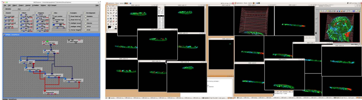
Figure 2: Illustrating the DDR system on a shared memory multiple GPU system employing a non-parallel file reader, and then parallel volume cropping and isosurface modules to form a visualization network using 20 DDR MPI processes. Usually the 20 sub-images are not displayed but, in this case, all images are shown as well as the final composited image that is visible at the top right. The network shown on the left is the visual programming interface for AVS/Express, which shows how relatively simple a parallel rendering application can be constructed by a non-technical user.
