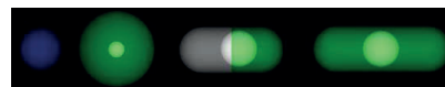
Figure 4: Effect of polarity: NaCl (ionic, left), HCl (polar, covalent, middle), \text{Cl}_2 (non-polar, covalent, right)
