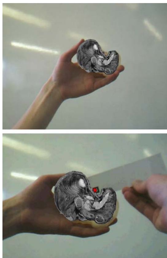
Figure 4: Showing the anatomy overlaid on the video image (top), and the resection tool in action (bottom)
