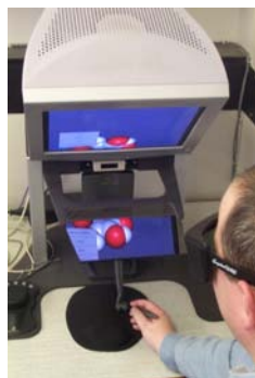
Figure 1: Molecular Visualiser. A stereoscopic projection of the molecule is co-located with the haptic device.
