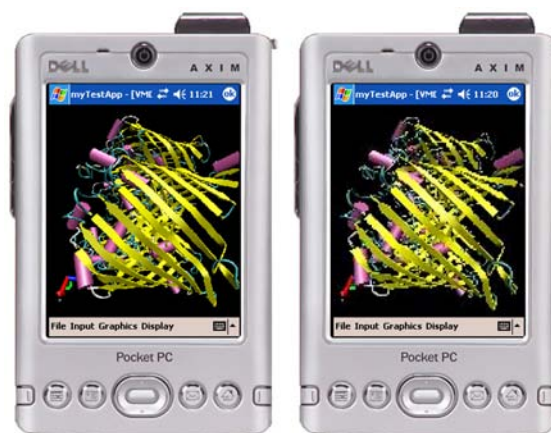
Figure 4: Adaptive frame encoding in Lightweight Visualization: lossless (left) / lossy (right).
