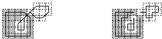
Figure 2: Example of overlapping contours: part 1. The first image shows two overlapping eight connected contours, while the second image shows the same image having to be represented as three four-connected contours.
