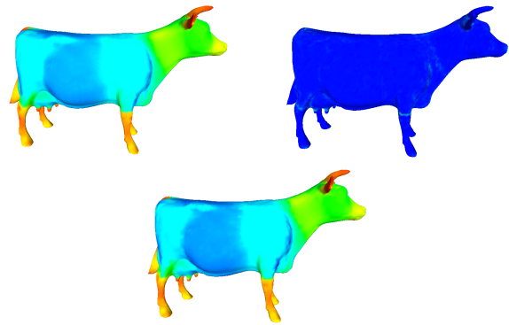
Figure 9: In this picture you can visually appreciate the difference between the SDF computed on all the faces and a subset (10% of the total number). The image on top left represents the result of the computation of the SDF on all the faces, while the one in the bottom represents the results of the computation performed on only 10% of the faces. In the top right image, the differences between the two results are graphically mapped on the mesh, with blue indicating no difference and colors towards red indicating larger and larger differences.
