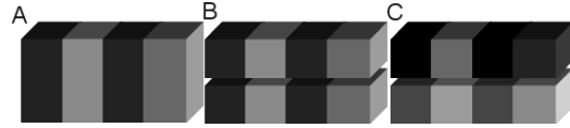
Figure 1: Slice splitting: original voxels (A) are subdivided in two parts with half z -component (B); the optimization procedure smoothing derivatives keep the sum of the original voxels unchanged (C).
