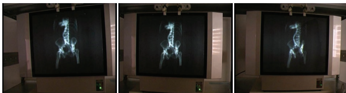
Figure 4: X-ray CT rendering. Direct capture from the spatial 3D display taken from different positions in order to immediately understand spatial information.
