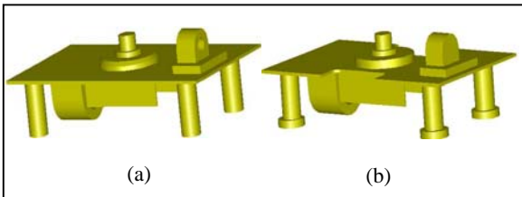
Figure 10 Adaptive simplified domain depending on the threshold value of accuracy: 10% for case (a) and 1% for case (b)
