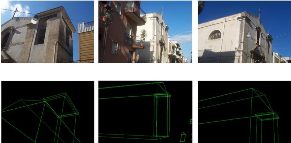
Figure 1: Some views of San Sebastiano's church in Carlentini; real (top) and reconstructed (bottom).
