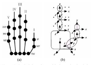
Figure 6: On the left, a schema of the human hand with the labels used to indicate fingers and joints. On the right the reference frames for the different joints are reported.
