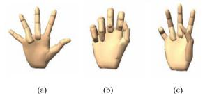
**Figure 5:** The effect of the calibration included in the CyberGlove software. The rendering in (a) corresponds to a user keeping his hand flat with the maximum abduction. In (b) the fingers should be clinched as a fist; in (c) the tips of little finger and thumb should touch.
