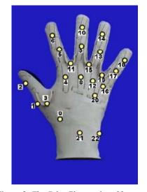
Figure 3: The CyberGlove with its 22 sensors.
