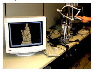
**Figure 2:** A picture of the system. The screen shows the virtual space in which the avatar, representing the fingertip of the user hand on the right, interacts with a sculpture.
