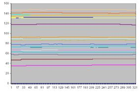
Figure 9: Output data sampled from the CyberGlove when the hand stands still on a flat surface.
