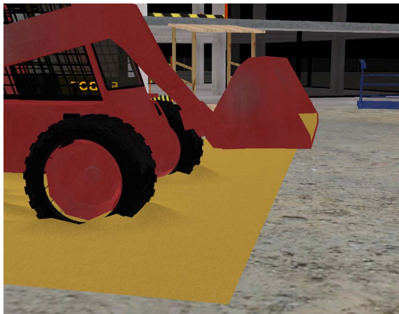
Figura 2: The interaction between terrain and other objects is simulated by a model based on terramechanics models.
