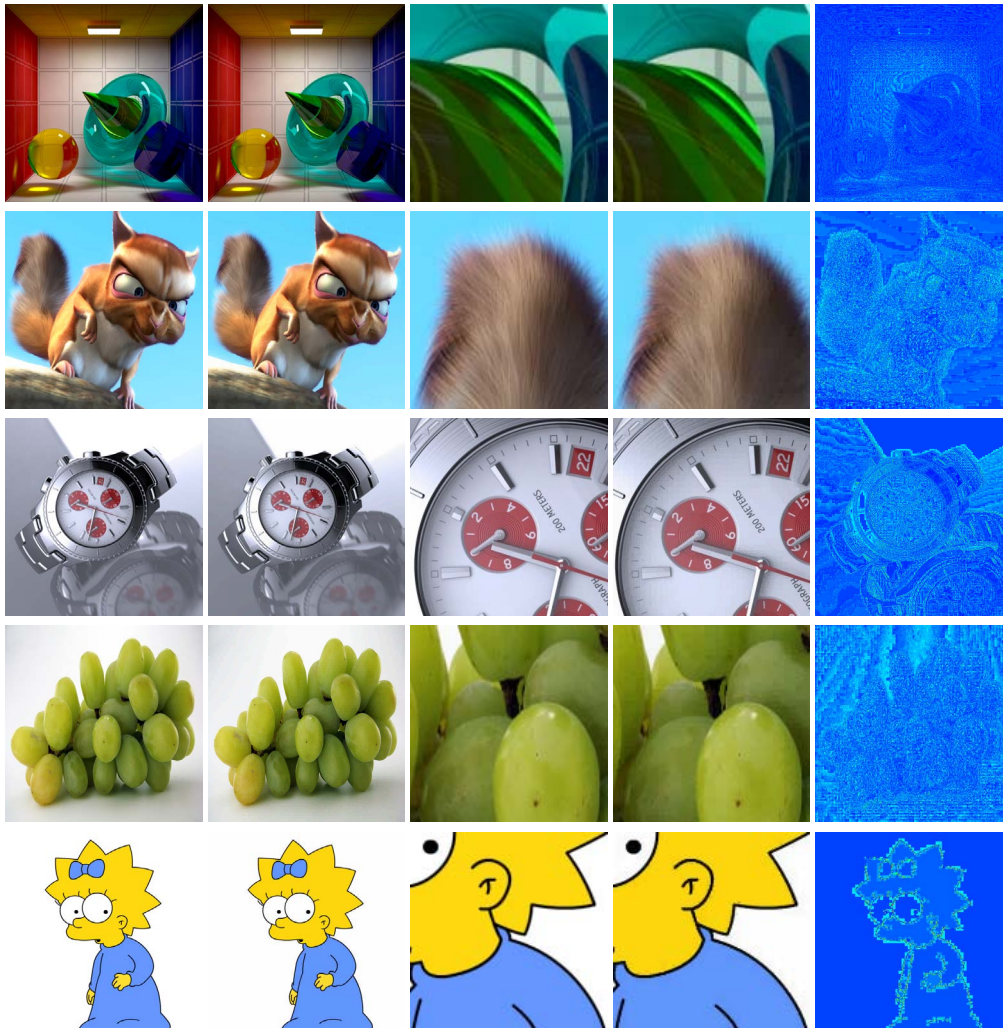
Figure 3: Compressed textures with rates varying from 6:1 to 24:1. From left to right: input image, reconstruction from our compressed representation, close-up views, and image difference amplified 10 \times .
