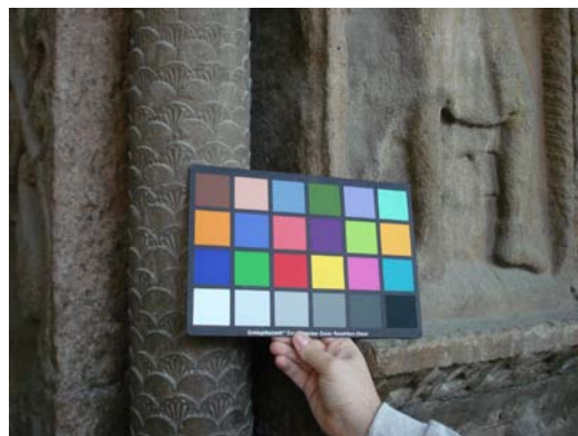
Figure 2: Color acquisition in Ripoll: color calibration for the photos.
