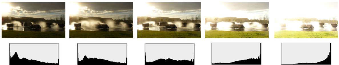
Figure 5: The complete bracketed sequence for the sunset scene, along with the respective histograms.
