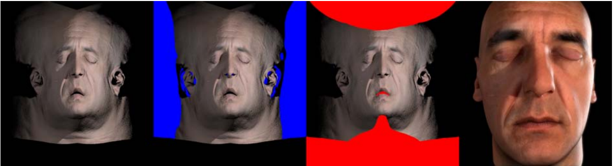
Figure 3: From left to right: irradiance map for a given viewpoint as described in [DLE07]. Culled and clipped irradiance maps: occluded and clipped pixels are highlighted in blue and red respectively for visualization purposes. Final rendered image.
