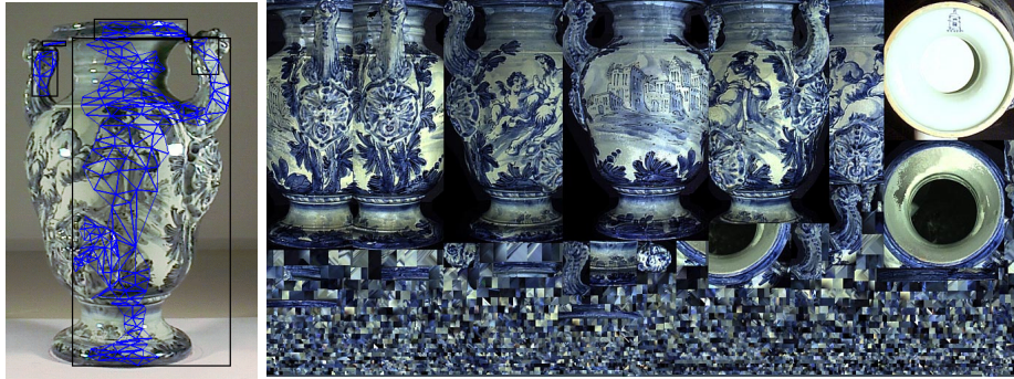
Fig. 8. On the left are shown (rendered wire-frame) the faces of M which are linked to a particular input image; in this case the corresponding texture section has an elongated shape, which can cause some space overhead in the final texture T_M (shown on the right).
