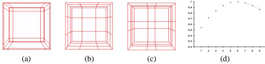
**Figure 4.** (d) Mutual information on vertical axis for an empty cube. Horizontal axis represents the relative displacement of a nearest subdivision to a common edge, ranging from 0 to 10. (b) corresponds to the optimal case, with value near to 6, (a) with value 2 and (c) with value 8.
