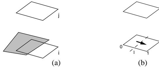
**Figure 1.** (a) Partially occluded patch pair. (b) (§4.2) Subdivision of a patch perpendicular to the radiosity gradient. The position of the cutting line is parametrized by the relative distance  $0 \leq l \leq 1$  to one edge.
