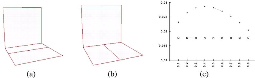
**Figure 2.** Mutual information on vertical axis (c) when dividing orthogonal (b,squares) and parallel (a,diamonds) to the common edge. Horizontal axis represents the displacement from the common edge (a) or one side edge (b).
