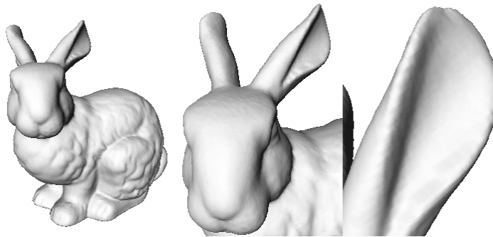
Fig. 4. All images show the isosurface at zero distance rendered with an inter-slice distance of one voxel. Note that the isosurface won't be hit exactly, but that we can arbitrarily decrease the inter-slice distance in order to get more accurate results.
