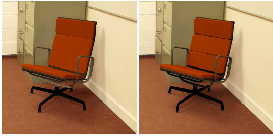
Figure 1: Interactive shading and shadowing of a 2,500 triangle synthetic object into a background photograph, running at over 11 frames-per-second on an NVIDIA GeForce4 GPU (left). For comparison, a ray-traced image is also shown, rendered in 1 hour using existing differential rendering algorithms (right).
