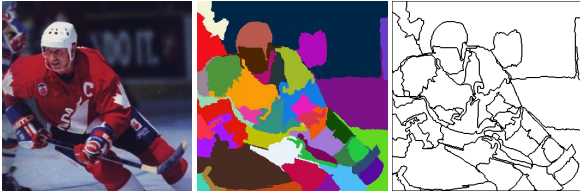
Figure 3: The original Gretzky image, left; the segmentation, centre; and the region boundaries, right.
