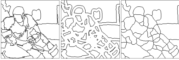
Figure 1: Region smoothing. Original region boundaries, left; the eroded region boundaries, middle; and the completely opened regions, right.
