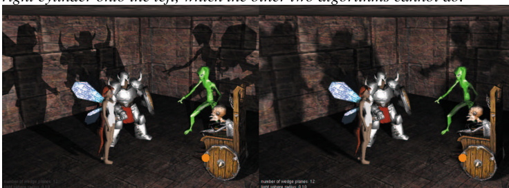
Figure 15: Rendered at 5 fps on a 1.5 GHz PC with a Geforce3. We modified nVidia's shadow volume demo (left) to render soft shadows (right).
