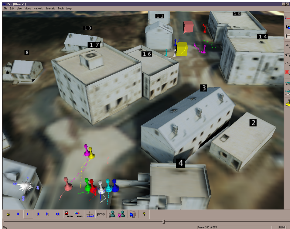
Figure 12: Moving objects detected in 3D and rendered as icons representing people and vehicles, rendered with the flashlight browser. Each object is color-coded with a unique color and its track over time is also shown.
