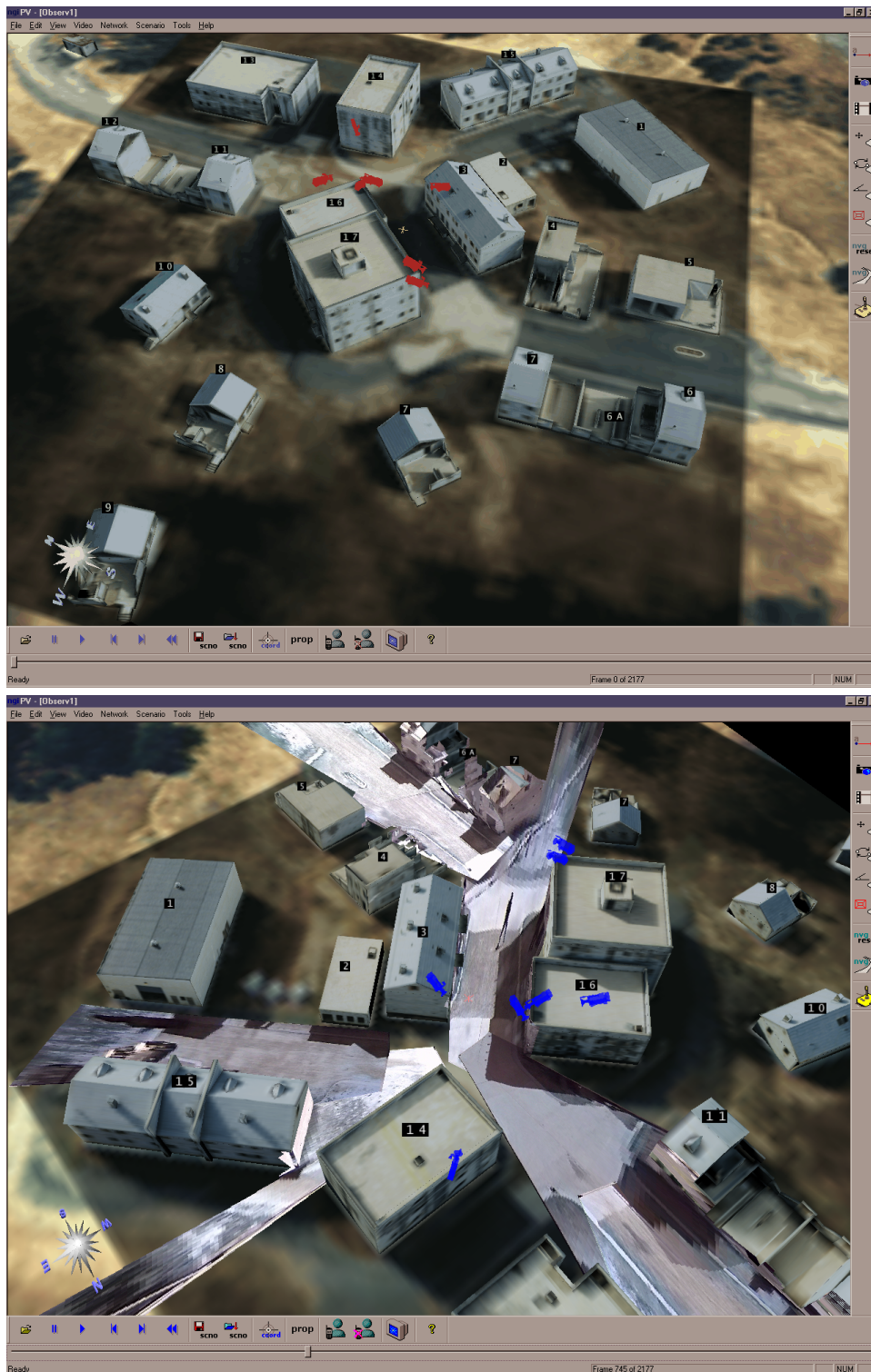
Figure 5: Video Flashlight Rendering: Top: A rendering of a textured model of a site with the location and orientation of video flashlight cameras shown in red. Bottom: Rendered view of the textured model and flashlight camera textures for 7 cameras rendered from a virtual viewpoint. The rendered view shows the effect of "illuminating" the scene with live cameras by "switching" on the cameras. The switched on cameras are shown in blue.
