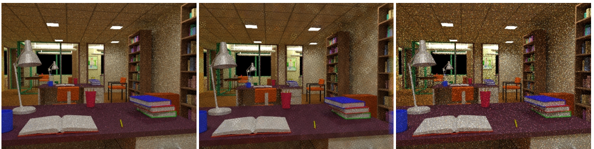
Figure 8: Left: image obtained with 160 paths per pixel, not re-using paths. Middle: 12 paths per pixel, with path re-use. The parameters are the same as in figure 7. The computation time was about 12 times lower than for the left image. Right: 12 paths per pixel, not re-using paths. We estimate that the speed-up caused by re-using paths is about one order of magnitude.
