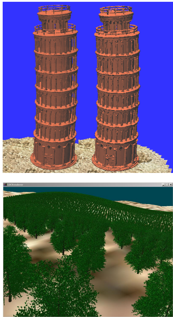
Figure 9: Top: comparison of Gaussian elliptical splats (left) with opaque squares (right) at splat size=2. Bottom: 50x50 non-compact objects (trees).
