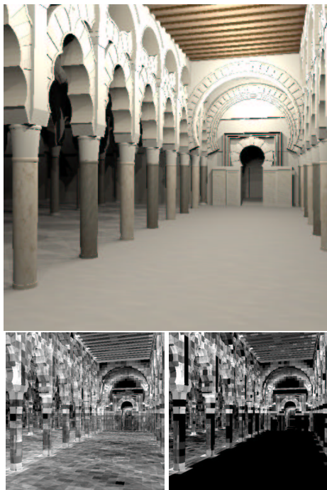
Figure 4: Top: Image of Mosque de Cordoba scene. Bottom left: Cost to render each pixel without masking (whiter is more expensive). Bottom right: Cost to render each pixel with masking.
