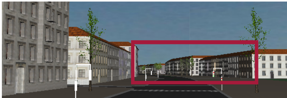
Fig. 1. A scene from an urban walkthrough. Geometry in the red region has been replaced by a point-based impostor, providing for fast, antialiased rendering of the far field.
