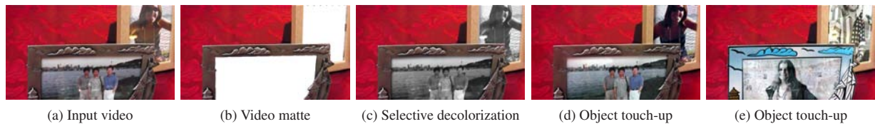
Figure 9: Video editing examples: Using the depths generated for the input video (a), and a user-drawn object-matte in a single video frame, the system can produce an object-matte for the entire video (b). (c) The object-matte can be used for a variety of effects like selective decolorization. (d) Any touch-ups made to an object in one or more video frames can be consistently applied to the entire video; in this case, reflections on top of the photos are removed. (e) Our system can also apply touch-ups to an object while preserving the lighting effects exhibited by the original object; in this case, the photos are changed without modifying the reflections.
