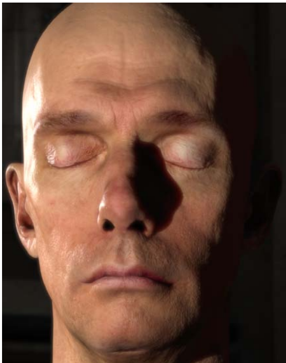
Figure 8: Real-time rendering with two point lights, one environment light, 16-bit floating-point buffers for high dynamic range, and two separable bloom passes.
