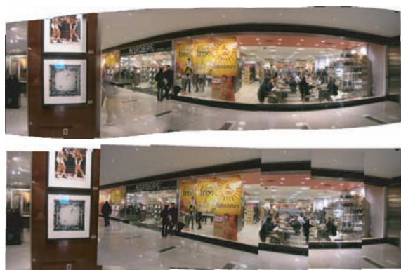
Figure 13: In this example, the seamless mosaic on the top obtained using image stitching may be considered to be more appealing than the scene collage with opaque layers at the bottom.
