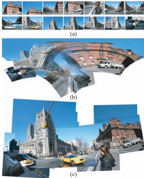
Figure 4: Comparison between scene collages and seamless panoramas. (a) Samples of 15 images as one crosses a street of about 25 meters wide. (b) A panorama obtained by applying image stitching to the set of images. This panorama is severely blurred in several areas due to significant parallax caused by the camera movement. (c) An opaque collage computed from the same set of images. While the collage has many boundaries, each of its components is perspective and the spatial arrangement of the components conveys the structure of the scene and the viewpoint movement. Compared to seamless panoramas, scene collages have boundaries (seams) but do not have distortions between the boundaries and are more tolerant to parallax effects.
