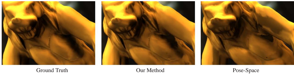
Figure 5: Another comparison between our interpolation scheme and pose-space based transfer matrix interpolation in the self-occlusion area. Pose-space interpolation fails to capture some self-occluded effects and has more visual artifacts
