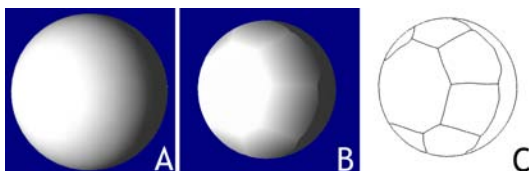
Figure 1: A: original bitmap; B: vector approximation (8 primitives with linear gradients); C: the primitives.
