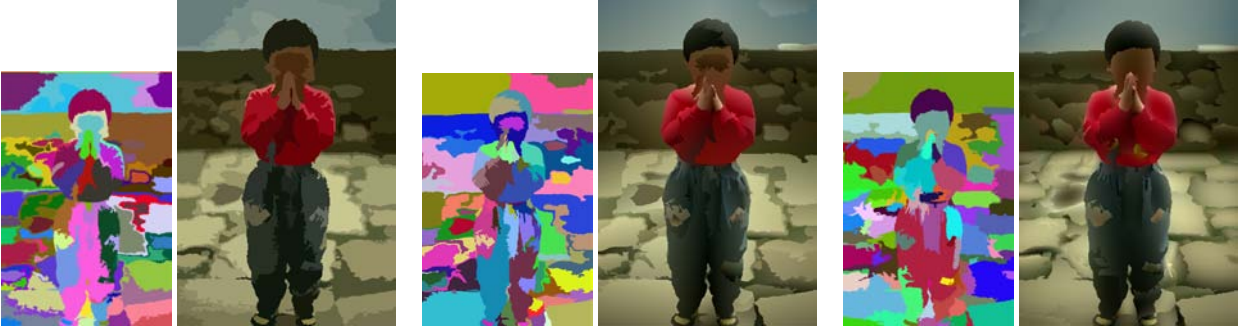
Figure 4: Segmentations and image approximations obtained with the pixel-based Ardeco algorithm, using regions of degree 0, 1 and 2.
