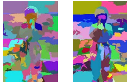
Figure 7: Left: Result of the two-level algorithm, obtained in 24 s. Right: The pixel-based version took 187 s on the same image.
