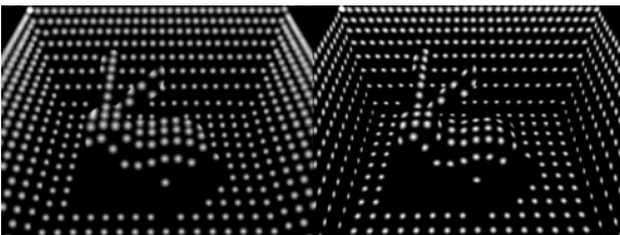
Figure 6: Sprite rendering: The images show light patterns generated by a few photons. The difference between screen-aligned textured point sprites (left) and the sprite-based ray-caster (right) is shown.
