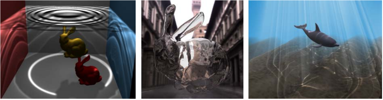
Figure 1: GPU photon tracing can be used to simulate a variety of different light effects at interactive frame rates. Even the rightmost scene including a dynamic object, shafts of light and caustics shadowing still runs at 10 fps on a 800x600 viewport.
