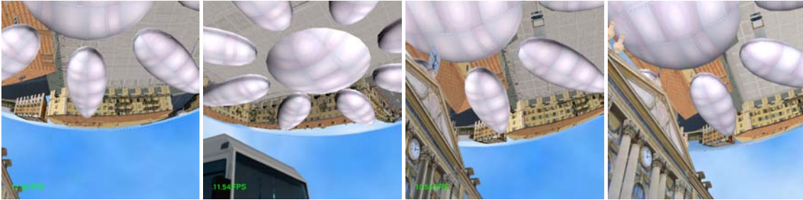
Figure 7: (Left) Three frames of the UFO scene (12 fps; 81,997 vertices). (Far right) Ray-traced image for comparison.
