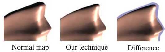
Figure 6: Comparison of normal-map with our technique. With an identical normal-mapped mesh and our outer hull, these two techniques produce identical results within object silhouettes; the only difference is that our technique correctly renders the silhouettes. The right-most image indicates differences in gray; as shown, all differences lie on the silhouettes.
