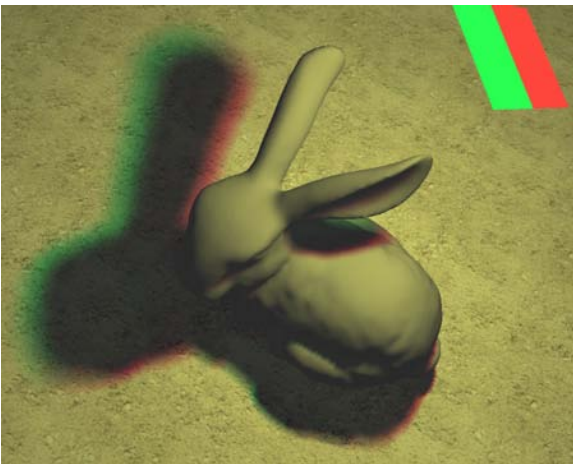
Figure 4: Soft shadows from a simple textured light source. For this example we have used the SAT option.
