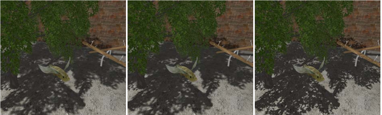
Figure 8: A scene composed of 800k polygons (screen resolution: 768×768 pixels). From left to right: reference image obtained from the average of 1024 light samples (17s per frame), our algorithm without adaptive resolution (23 fps) and standard shadow mapping with hardware 2×2 percentage closer filtering showing the pixels of the shadow map (40 fps).
