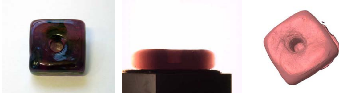
Figure 1: Left: glass object. Center: one of 360 input images. Right: reconstructed geometry, including some left-over support structure that the object was placed on during acquisition. The reconstruction is the raw output of our method, without further processing.
