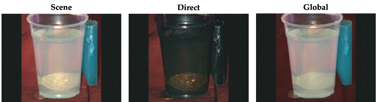
Figure 6: Plastic Cup with Milky Water and Coin: In this example, the global image includes the volumetric scattering [Cha50] [Ish78] of light by the milky water (referred to as "airlight" in atmospheric optics [Mid52] [McC76]) in the cup as well as the secondary illumination of the copper coin by the milky water [SRNN05]. The direct component includes the specular highlights on the copper coin due to direct illumination of the coin by the source. This component is attenuated (referred to as "direct transmission" in atmospheric optics [Mid52] [McC76]) by the milky water as it makes its way to the camera. The wax candle on the right has a strong subsurface scattering component. As a result, all of its color is captured in the global image and the direct image only includes the surface reflection (highlights) from the candle.
