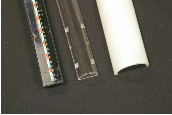
Figure 3: Left: opened iColor Cove light source. The left side of the circuit board is already covered with reflective foil. Center: clear cover for the light source. Right: diffuser built from acrylic tubing and white spray-paint.
