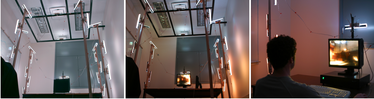
Figure 11: Left: photograph of the room housing our system, with all lights switched on. Center: illumination programmed to resemble the Grace Cathedral environment. Right: A user viewing the Grace Cathedral environment on an HDR display in a room illuminated by our system. Note how the room illumination is consistent with the virtual environment shown on the screen.
