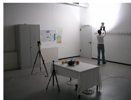
Figure 5: Measurement setup for the still camera: an Olympus C5050Z digital camera records objects on a table which are indirectly lit by a hand-held spotlight pointed at the white walls, ceiling and floor. The probe object, a black snooker ball, is mounted on the small tripod next to the table.
