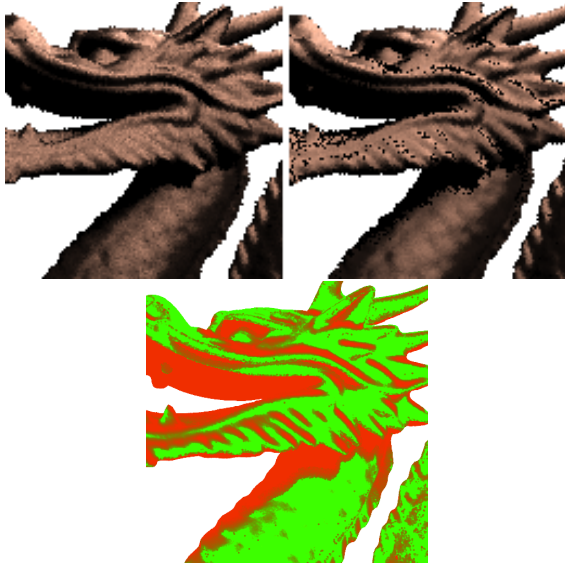
Figure 3: Dragon sampled with a single primary ray and using RIS with different values of M and N to compute direct lighting (in equal time). On the left, N = 20 , M = 1 and on the right N = 1 , M = 60 . The right image has less variance except where visibility is a major component of the variance. The lower image shows the optimal ratio of M and N . Green (lighter) pixels correspond to larger M , red (darker) pixels to larger N .
