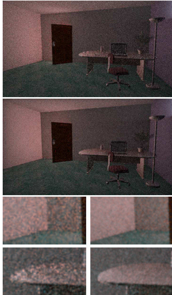
Figure 3: An example of variance control due to the user path proposal strategy. Top is the image rendered with no user paths, while center is the result when the user specified ten paths passing through the doorway. Bottom are zooms of the wall intersection and table regions, with no user paths on the left and user paths on the right. These are MLT images that directly visualize the sampled light paths. The improvements after a final gather, while present, are less apparent.
