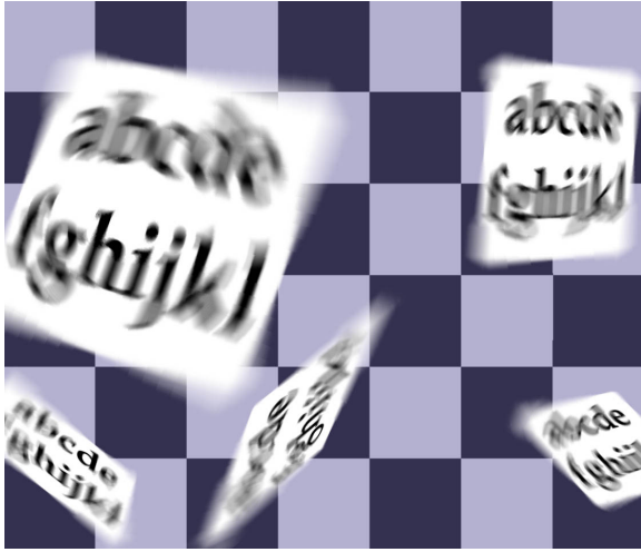
Figure 3: Tumbling billboards and other typographic animations profit from motion blur of the textures. The geometry to which the textures are applied extends beyond the billboards, which are formed by the texture’s alpha channel.
