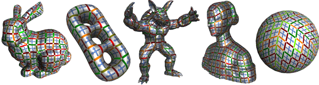
Figure 7: Sign assignment and tile arrangement on models (left-to-right): BUNNY, HOLES, ARMADILLO, LAURANA, and a quad-based icosahedron (mapped on a sphere). The arrows on tiles indicate the associated signs and cycle directions.
