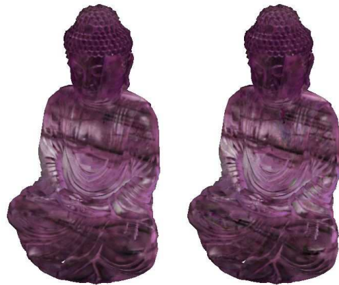
Figure 8: The buddha model processed using PCA, on left, and the Online SVD, on the right. Online SVD is an approximation, and there are some visible artifacts in the chest area. The PSNR between the images is 33.2dB.
