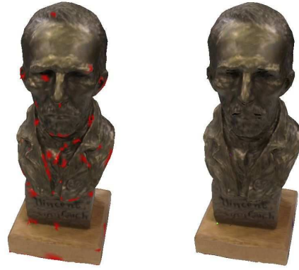
Figure 5: The left image shows the bust model constructed from 282 pictures, and the right image shows the same set of images using imputation to fill in the missing values. Areas with missing data have been colored red (they would normally be black).
