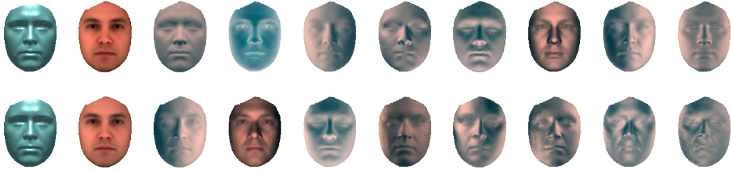
Figure 5: The illumination bases of 9-D using nine harmonic images (upper row) and our bilinear model (bottom row) for a certain 3D face model with average shape and texture. Each base is scaled independently to cover the full color range for purposes of visualization.
