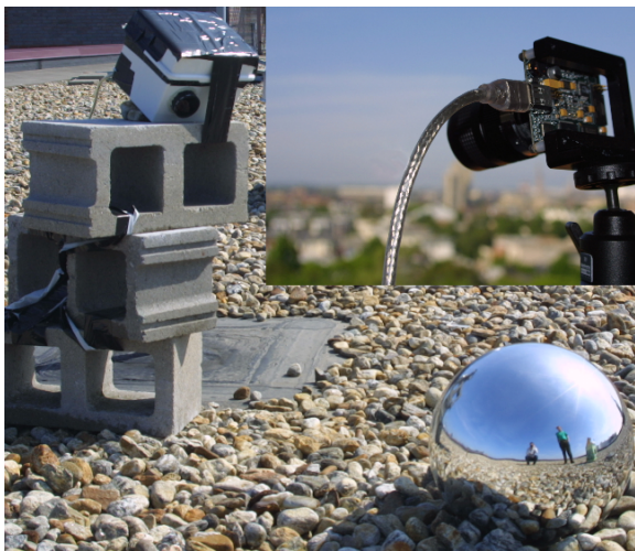
Figure 5: Acquisition system for an outdoor (city) scene.
